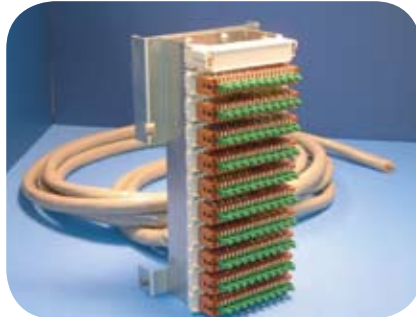
Typical Factory Preterminated xDSL IN/OUT Block with 10-Foot Stubs, Rear Exit (100-Pair Shown with JMS Bracket Installed)
