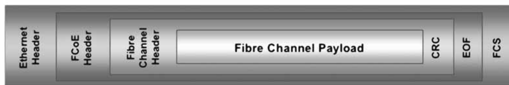
Figure 1 – Ethernet Encapsulated FCoE Frame
