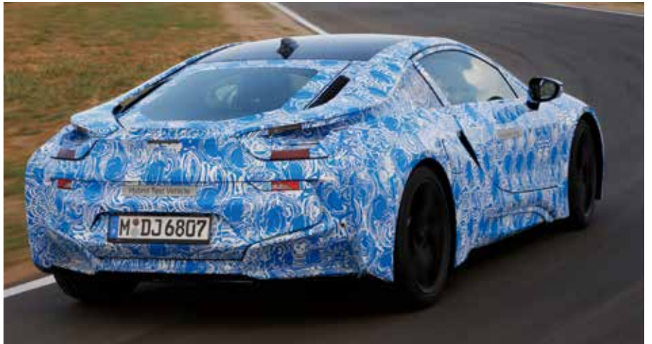
The new BMW i8 is the first production car with Gorilla Glass, used in the rear windshield.
