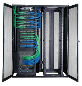
EN Enclosures are designed so that the front doors open to the left or right. When two enclosures are ganged together, doors can open in opposite directions, creating a large space where cables are easily accessible and able to be routed up, down, or to the next enclosure.
