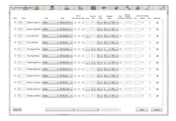
The **Common Configuration** screen shows all of the connected Devices. Depending on the number of devices that need to be changed you can use the "**Select all Button**" to select all the Devices and then deselect the devices you don't want to change or you can select the Devices you want to change by clicking on the Select box next to each Device.
