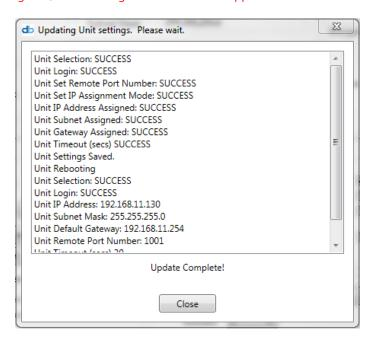
When the Device unit upload is complete, a confirmation message appears. The status window can be closed and Device unit data entry continued.
