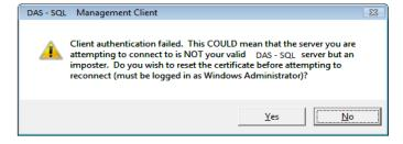
If the User knows the server's certificate has changed, and trusts the server, the server certificate identifier on the client can be reset to accept a new certificate from the server. To do this, click the "Yes" button on the message box.
