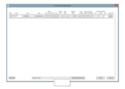
Multiple settings can be changed for selected Device(s). Click the Left Combo Box, select setting to change, Click the Right Combo Box to select the new value setting. Click the "**Set Selected Device**" button. Now click the Left Combo Box again and select a different setting to change, set the value, click "**Set Selected Devices**" button. After all the settings that need to be changed are entered Click on the "**Save**" button and the new changes will be transferred to the Devices.
