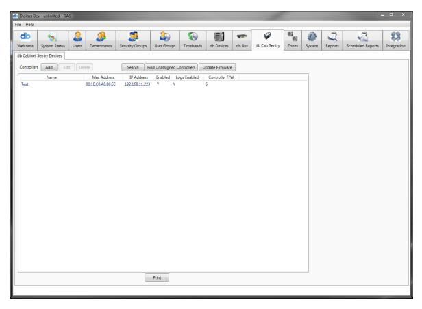
Currently configured Devices are shown in the "Devices" list. This list can be sorted by Name, IP Address, or Zone. To sort the Devices, left-click on the column header.
