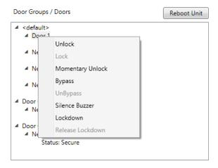
To send a command to the Device, select the command from the menu. It normally will take less than two (2) seconds for a command to execute and the new status will be displayed for the affected Device. An "Action Request By User" transaction will appear in the "Events" list, followed by the appropriate "Unit Event" when (and if) the requested action occurs.
