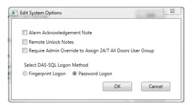
**Alarm Acknowledgement Note** - Works with the System Status tab and Alarm events. If selected, the operator will be required to enter a note when acknowledging alarms that have occurred in the system. These notes are stored in the database and can be reviewed via a report run from the reports tab.
