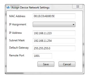
This form allows the Device unit's network settings to be reconfigured. The network adapter in the Device can use a fixed (static) IP address or an automatically assigned address (DHCP). Note that if "Automatic (DHCP)" is selected, the unit will receive an address assigned by the network DHCP server, but the IP address (the '...' address) must be used (not a "computer name").
