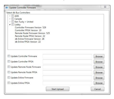
This window shows the current firmware version of the db Bus Controllers in the system. To update the controller's firmware, select the controller to be updated, select the relevant components by checking the checkboxes next to each item, and then browse to the relevant file. Once everything has been selected, click the "*Start Upload*" button. A progress and percentage image will show the update's progress.
