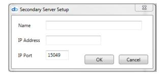
Within the Add window, create a Name and add the IP address and Port that DAS-SQL will use to communicate with new server.
