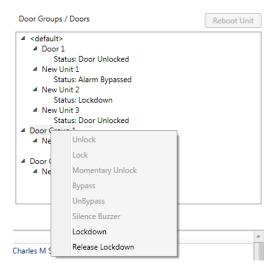
To send a command to the Zone, select the command from the menu. It normally will take less than two (2) seconds for a command to execute and the new status will be displayed for the affected Device(s). An "Action Request By User" transaction will appear in the "Events" list for each Device, followed by the appropriate "Unit Event" when (and if) the requested action occurs.
