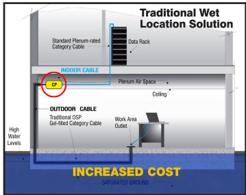
Outdoor (non-rated) cables are often used for below grade and in-the-slab applications. In these instances, the outdoor cable must transition to the appropriately rated indoor cable, such as plenum or riser, upon entering the building interior. This method of using two types of cable requires additional materials and labor as well as space for the consolidation point (CP).
