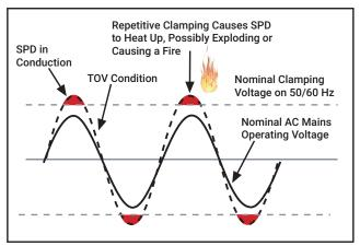
To meet the fundamental requirements of performance, longer service life and greater safety under real world conditions, nVent ERICO has developed Transient Discriminating (TD) Technology.
