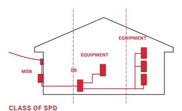
In the IEC system, SPDs are tested to various Test Classes, intended to assess and assure their suitability for use in different locations and circumstances. Strictly speaking, the Class refers to the type of test, not to the SPD. However, in common usage, SPDs are referred to by their Class, For example, a Class I SPD is an SPD that has been tested to Class I requirements (of a specified severity), and so on.
